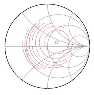
Figure 13. Load match contours for constant delivered power
