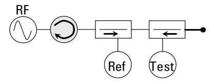
Isolators are typically narrowband devices. If an isolator is used in an X-parameter measurement it may not be possible to stimulate the DUT with harmonic extraction tones, however, useful X-parameter information may still be extracted. For example, power supply sensitivity, compression, DUT harmonics, and fundamental match measurements may result in a useful model for simulation.
