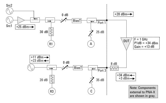
Figure 3. +34 dBm amplifier setup
