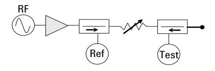
When measuring low gain devices, a pre-amplifier may be added to PNA-X port-1 to increase the DUT input power. As a general rule of thumb, the preamplifier's harmonics should be about 20 dB below the maximum main tone at the DUT input to avoid stimulating nonlinear behavior in the DUT which cannot be corrected by the NVNA.
