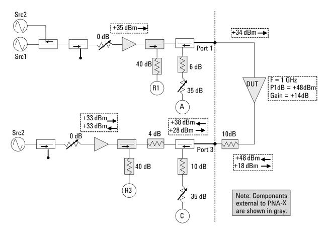
Figure 4. +48 dBm amplifier setup
