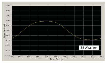
Figure 8. B2 (DUT output) waveform versus time, at 200 MHz, Pout = +50 dBm
