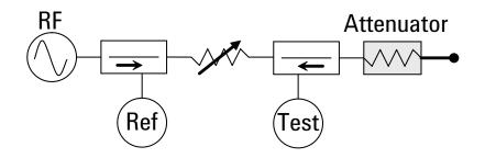
The cable connecting the attenuator to the test port should be kept as short and stable as possible to minimize directivity drift.
