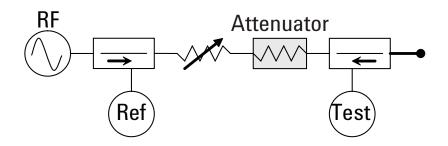
The cables connected to the attenuator should be kept as short and stable as possible to minimize measurement drift.
