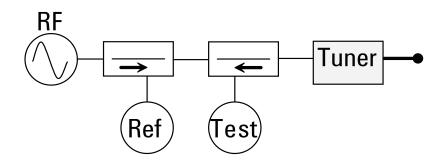
The tuners are placed directly at the ports of the DUT in order to provide the widest range of load conditions possible. If low loss couplers are available then the couplers can be placed between the tuner and the DUT.
