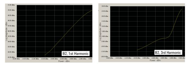
Figure 10. B2 (DUT output) power out versus power input, at 200 MHz for 1st and 3rd harmonics
