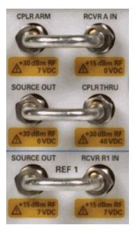
Figure 2. PNA-X N5242A port 1 front panel jumpers
