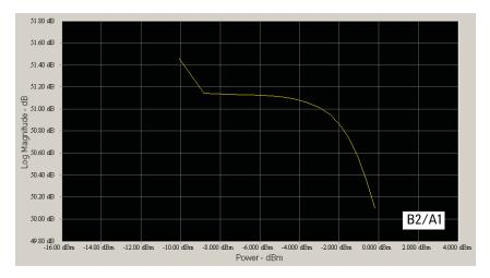
Figure 9. B2/A1 (DUT gain) versus power input, at 200 MHz for 1st harmonic
