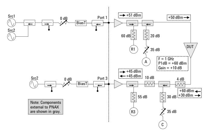
Figure 5. +60 dBm amplifier setup
