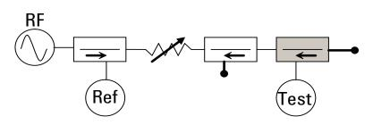
Note that the PNA-X test coupler arm rolls off at 20 dB/decade for frequencies below 700 MHz, so that the typically -15 dB coupling factor is reduced to -52 dB at 10 MHz. If an external test coupler is added which doesn't exhibit this roll-off, then the dynamic range at low frequencies will be improved.
