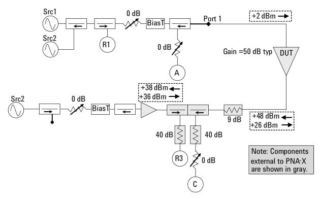
Figure 6. 100 Watt amplifier setup
