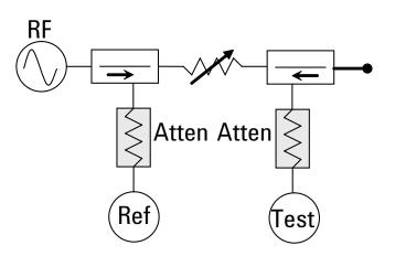
The PNA-X has an internal transfer switch located between the R1 receiver and the coupler arm. When adding a pad to the R1 receiver path, ensure that the internal transfer switch has been set to the "external" mode so that the pad is included in the measurement path.
