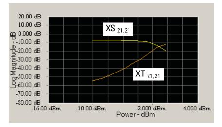
Figure 11. XS<sub>21 21</sub> and XT<sub>21 21</sub> versus power input at 200 MHz
